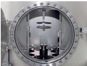
Used chamber enables comparison in vacuum of maximum 10^{-6} mBar or in noble gases such as argon.
