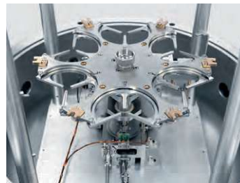
The mass comparator features magazine for 6 cylindrical objects of \varnothing(22 - 95) \times 110 mm or sphere objects of maximum diameter of \varnothing 100 mm.
