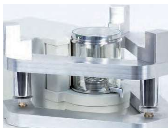
The modular design enables to use the susceptometer as a microbalance or a mass comparator.
