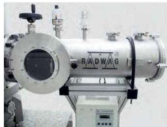
The LOAD LOCK system for transfer of mass standards enables switching and adding artefacts without changing the atmosphere inside the main chamber.
