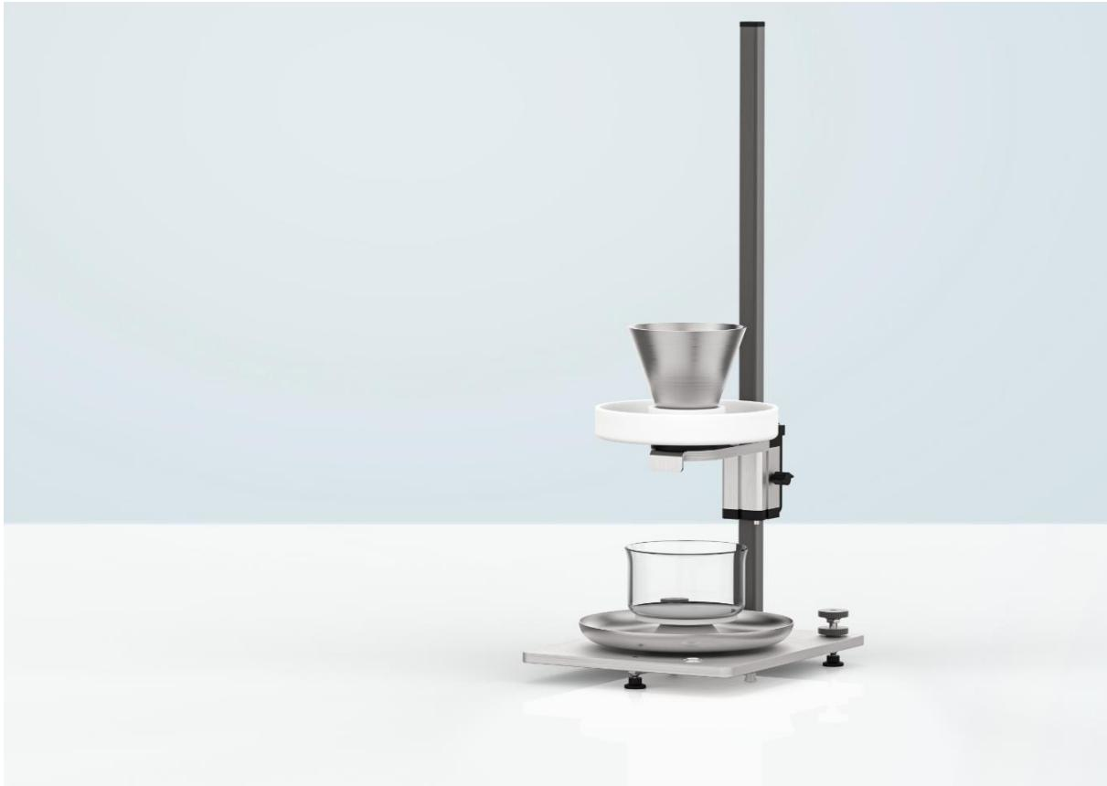
To measure the flowability, a stopwatch and a laboratory balance are used to check the time it takes for 100g of sample to flow through the funnel and to be collected inside a plastic beaker. Changing between these modes of operation is easy and does not require the use of any tools.
