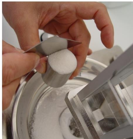
The PT-SV110 is easy to use. First weigh then place the stainless steel cup onto the base of the unit. Then carefully pour the powder into the funnel at the top of the baffle box until the cup beneath overflows. Now level off the powder using a flat edge scraper.
