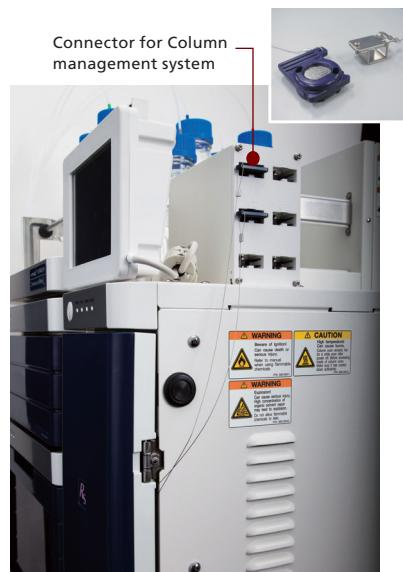
A view of connector for column management system connected
