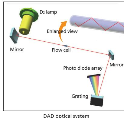
A quartz glass capillary tube is adopted as the flow cell channel, and the efficient total reflection at the capillary surface is harnessed to minimize the loss of flow cell transmission light. Consequently, even with the elongated optical path length of the flow cell, the baseline performance is comparable to the previous flow cell, resulting in a sensitive detector.
