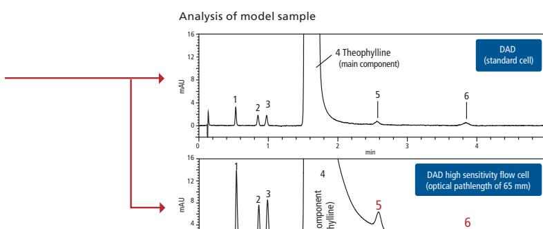
The use of the high sensitivity flow cell demonstrates reliable detection of the related substances (0.005% each).
