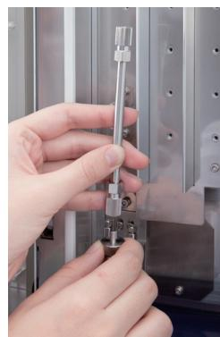
A view of operation of attaching a column
