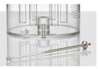
Use a printer which is connected to the PTZAUTO to get a printed report. If the SPT-6 is used with the PTZS Disintegration Test Apparatus the operator has to record visually the time and calculate any statistic. There will be no automated print-out. The supply scope of the SPT-6 Test Assembly includes a round Plexiglas water bath including tubing connectors to attach the bath to the heating system of the disintegration tester.
