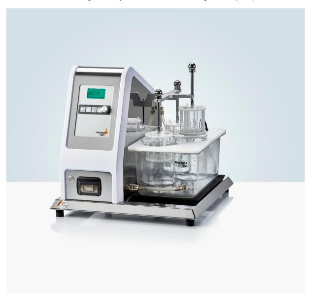
Tablet disintegration testing instruments are widely used in the pharmaceutical industry to evaluate the disintegration characteristics of formulations and the quality control of different dosage forms. All Pharma Test tablet and capsule disintegration testers are fully compliant with the current USP and EP Pharmacopeia and support both A-type and B-type baskets for regular or larger samples. They
