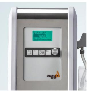
Access to the instrument is protected by a login with username and password. Optionally a quick test menu can be accessed without logging in to the instrument first. This way tests can be performed with the instrument in case user access control and testing according to defined methods is not required.
