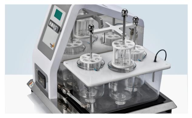
The disintegration basket which holds the glass tubes and discs, is placed into a metal holder and held by a magnet. The instrument detects if a basket is inserted or not. The illuminated LC-display shows status information, like the elapsed testing time. The disintegration basket is moved up and down by 55mm (each way) at a rate of 30 times per minute. At test start it is moved smoothly into the testing medium.
