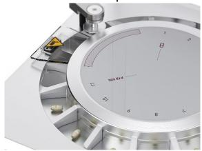
PTB 500 features a carousel to transport the samples between the weight, thickness and combined width, diameter (or length) and the hardness testing station. It features and integrated Sartorius analytical balance to measure the weight of the individual samples. The measuring units can be selected from mm or Inch and KP (Kilopond), N (Newton) or Sc (Strong Cobb).
