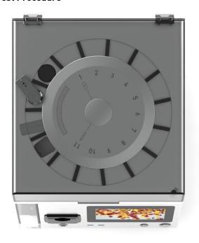
The samples are automatically transported to the test stations by the rotating carousel. First the weight is measured by the integrated Sartorius analytical balance. Then the thickness is measured and third comes the combined diameter (or length) and hardness testing station. It is also possible measure the width of the sample. In this case the operator is prompted to position the sample accordingly in the test station.
