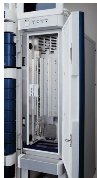
A view of column oven accommodating columns
