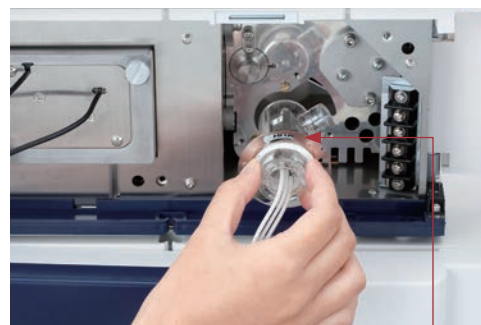
Front access (Example: replacing lamps)
