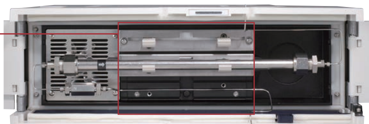
The photo represents a unit in which a part of the pre-heating cover is removed.
