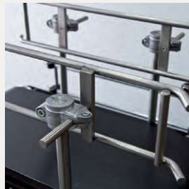
Conveyor side guides
