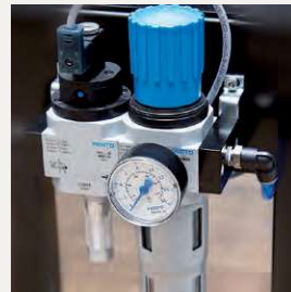
Compressed air service units
