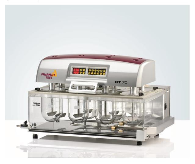
Tablet dissolution testing is one of the most important tests during development and manufacturing of solid dosage forms and Transdermals. Nearly all international pharmacopoeias describe a dissolution test instrument, in which at least 6 samples should be tested. The test vessel design, stirring speed range, temperature range and accuracy, stirrer design and relevant tolerances are specified.
