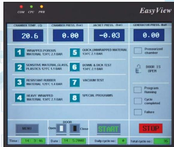
There are also two test programs which are: Bowie&Dick and vacuum leakage.
