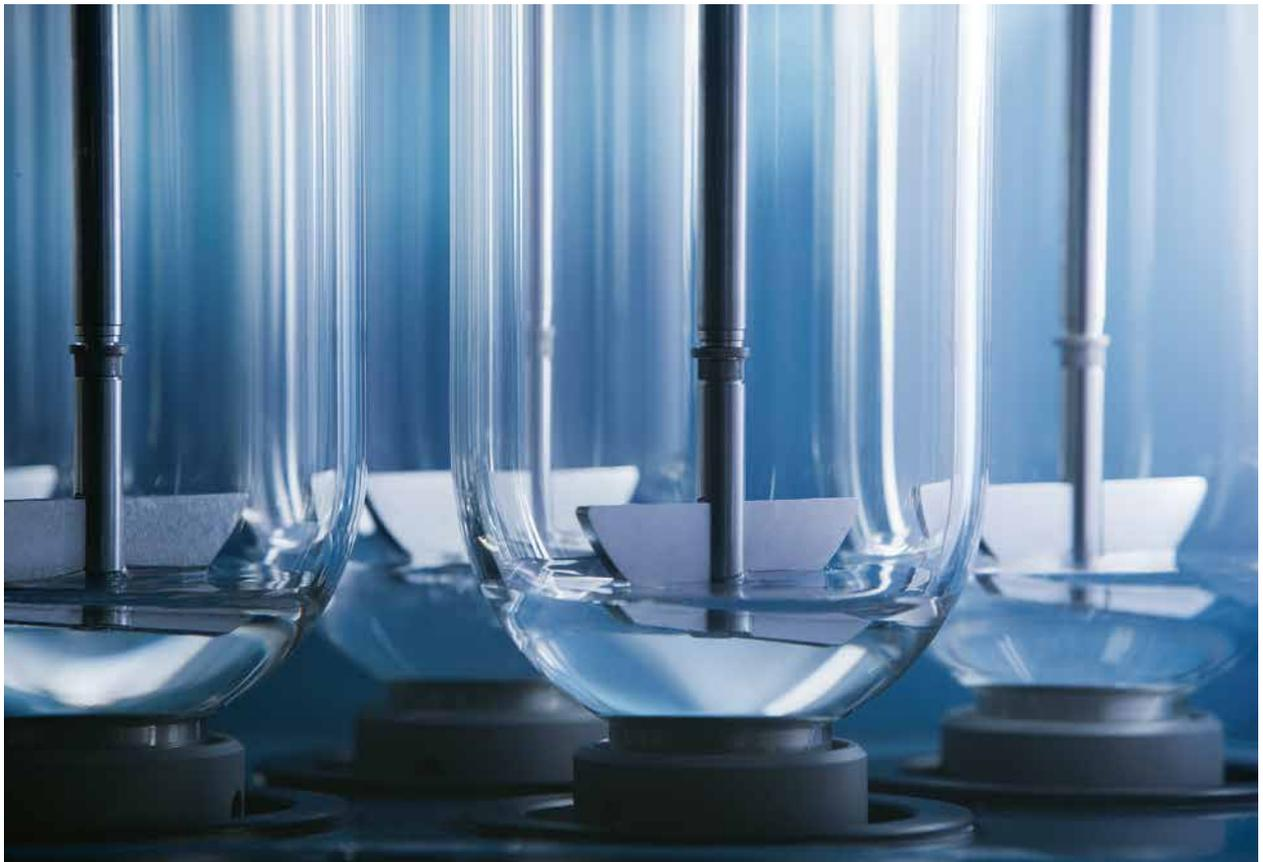
→ Simultaneous media dispensing into the vessels through the hemispheric valves
